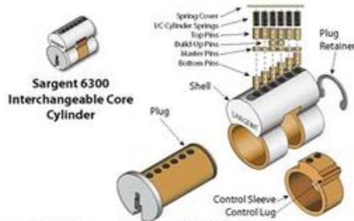
Figure 10.01 Sargent 6300 LFIC Cylinder
