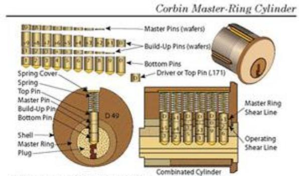
Figure 6.05 Corbin Master Ring Cut-Away View
