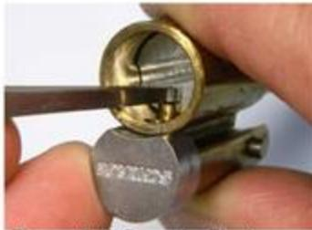
Figure 15.17 Press the Pin down
