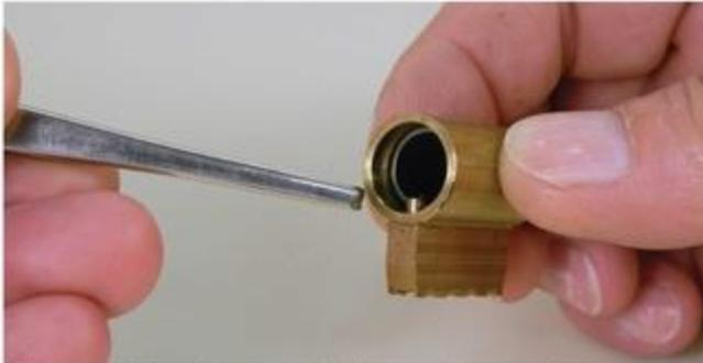
Figure 1.36 Top pin jammed, holding its cylinder spring compressed
